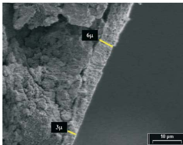
Figure 3. SEM photograph of the external surface of catalyst C3T (2000 \times ).
